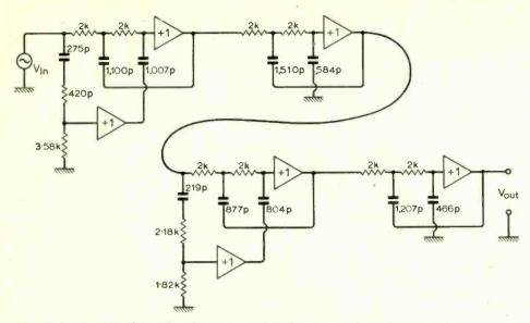
Fig. 19. Realization of the 8th-order Storey-and-Cullyer linear-phase characteristic. Resistors,  $\Omega$ . Capacitors, pF.
