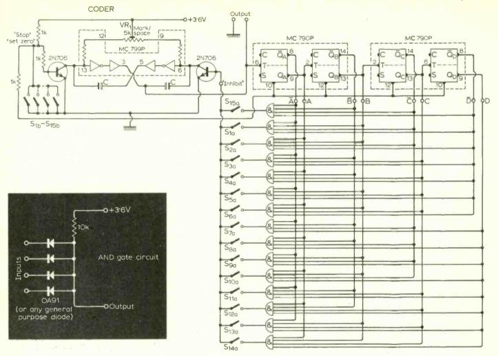
Fig. 3. The circuit of the coder (Above) and decoder (Below). If wished the decoder may be used with the relay decoding system of Fig. 2 or with the same AND gate networks as the coder. The inset above gives the circuit for the AND gates. A relay drive circuit for use with relay decoding and an alternative decoder input circuit for use with a relay input are given in the lower inset.
