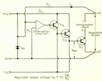
Fig. 2. Using a separate supply line for the stabilizer circuitry.
