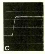
Fig. 16. Step responses of three filters: (a) a 5th-order Darlington, (b) a 5th-order Butterworth, (c) an approximate linear-phase filter.
