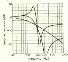
Fig. 5. Measured responses of the individual stages of a filter as Fig. 4, scaled to give —3 dB at 159 Hz.
