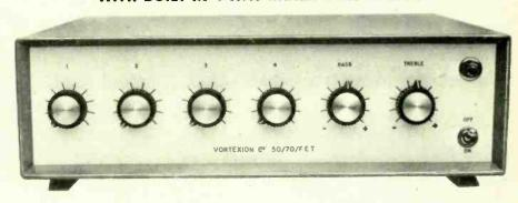
100 WATT ALL SILICON AMPLIFIER. A high quality amplifier with 8 ohms-15 ohms or 100 volt line output for A.C. Mains. Protection is given for short and open circuit output over driving and over temperature. Imput 0.4 V on 100K ohms.
