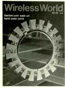
This month's cover illustration shows an unusual view of a watchmaker's wheel adopted by Pye to aid the handling of components in the production of small receivers (see p.158).
