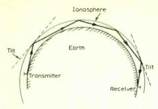
Fig. 6 Chordal hop. At the first and last reflection points, the ionosphere behaves as if tilted slightly towards the terminals. For tangential radiation (i.e. zero deg.), and tilt, however small, prevents a return to earth until a tilt of opposite sign occurs. (Ionosphere not to scale.)
