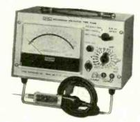
H.F. VOLTAGE RANGES 1 mV, 3 mV, 10 mV . . . 3V f.s.d. Square law scales. Acc.  $\pm$  4% of reading ± 1% of f.s.d. at 30MHz.
