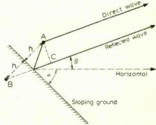
Fig. 2 With the aerial at a height h above ground sloping at an angle ∞, the direct and reflected waves are in phase when 2h  $\sin(\alpha + \theta) = \gamma \lambda/2$ . For small values of \(\theta\) this becomes 2h sin \(\pi \approx \approx 1/2\). This diagram is identical with Fig. 1 except for rotation through the angle a, and the increased ground angle.
