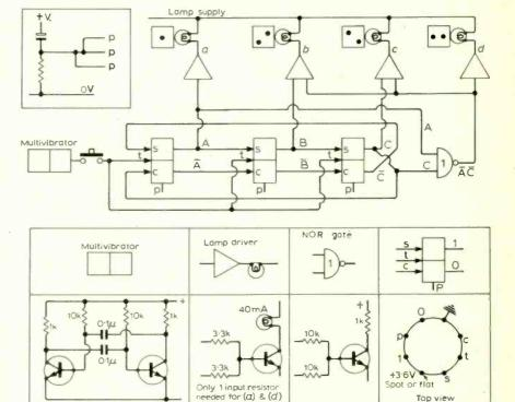
Fig. 2. The suggested circuit for a digital dice, the method of display is left to the reader, almost any general-purpose silicon transistors may be used.
