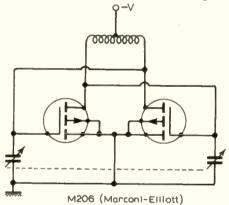
Fig. 1. Oscillator operating up to 300MHz.
