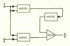
tronics. The inputs X and Y can be of any sign. Use is made of the fact that  $X \div Y = (XY)/Y^2$ .
