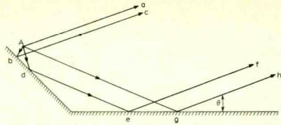
Fig. 3 Ground sloping down into the sea. The direct wave Aa, foreground reflection Abc, distant reflection Agh, and double reflection Adef add in phase if  $\theta$  is small, hg  $\approx \lambda/(4 \sin \theta)$ ,  $h_s \approx \lambda/(4 \sin \theta)$ , these being the heights of A above ground and sea respectively.
