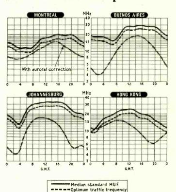
The predictions are based on an ionospheric index of 96, the corresponding sunspot number being 83. These are slightly lower than the observed values for 1968 and 1969.
