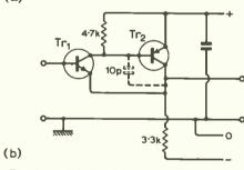
Fig. 14. (a) 3rd-order low-pass filter, -3 dB at 4.75 kHz. (b) Suggested amplifier.  $Tr_1$ : 2N3707, 2N3904, BC109C etc.  $Tr_2$ : 2N4058, 2N3906 etc.
