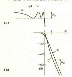
Fig. 15. Illustrating 5th-order Chebyshev response: (a) pass-band ripple, (b) increased attenuation compared with Butterworth 5th-order response, B.
