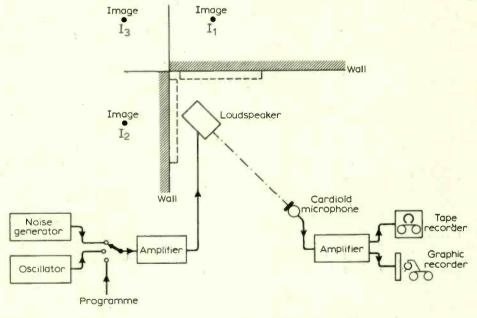
Fig. 1. Experimental set up used for investigating effects of corner placing.
