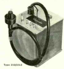
A compact oil filled ringing transformer/rectifier unit, supplying 25Kv. at up 30 350 micro amps, suitable for dust extractors, air purifiers, paint spraying or any application requiring a smoothed well regulated 25Kv.
