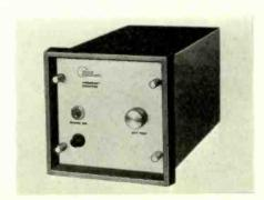
speed and overspeed modules can be housed in a single instrument to provide bandpass or high- and low-limit facilities. Thirteen overlapping ranges cover the frequency spectrum 1Hz to 30kHz. Alarm operation is within 0.1% of the set point and reset is automatically carried out without hunting. Output can be in the form of a relay changeover or of a logic level change. Construction is of i.cs mounted on plug-in p.c. modules. Orbit Controls Ltd, Alstone Lane Industrial Estate, Cheltenham, Glos.
