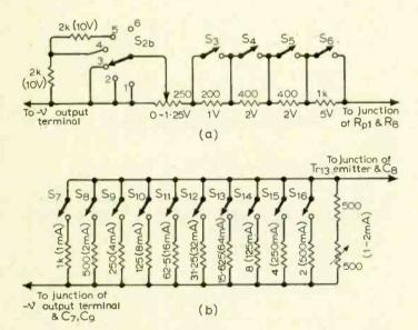
Fig. 9. (a) Construction of R<sub>V</sub>; (b) Contruction of R<sub>C</sub>.
