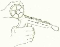
The first is called Tyton - an 'off-thereel' system that binds 50% faster than any other comparable system. The second is Kabelrap - a heavy duty version using 'one-piece' ties.
