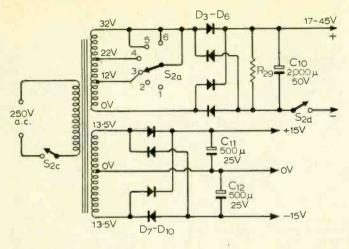
Fig. 8. The d.c. supply circuits.
