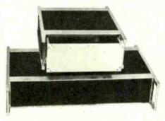
downwards or accidentally dropped. The protrusions at the rear which allow the case to stand face upwards, also protect rear connectors and components. The standard case, CS1 which is bench mounting can be converted to 19-in rack mounting simply by fitting brackets to each side. The CS1 will accept one module M1 or two modules M2. The CS2 or "half rack" case accepts one module M2 only. Case Systems, 20 Hunt Lane, Chadderton, Lancs.
