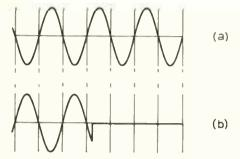
Fig. 6. Instead of switching on, as shown in Fig. 5, one signal is switched off.
