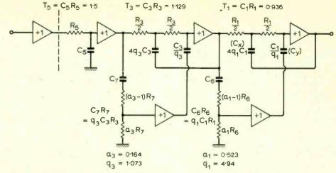
Fig. 4. Schematic for realization by factors of 5th-order Darlington response with 0·1 dB ripple in the pass band, 40 dB minimum attenuation in the stop band, and cut off at 1 radian/second.
