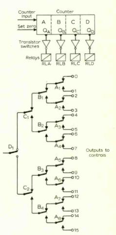
Fig. 2. (Above) Showing how the decoding can be performed with relays.
