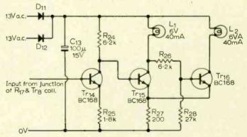
Fig. 7. Overload indicator circuit.
