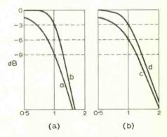
Fig. 17. Amplitude responses of Butterworth and approximately linear-phase filters.
