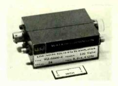
a guaranteed noise figure of 8.5dB maximum and power output of +7dBm (for 1dB gain compression). Overall design is consistent with the respective environmental requirements of MIL-E-16400F. Watkins-Johnson International, Shirley Avenue, Windsor, Berks.
