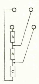
4-terminal connections minimise lead and contact resistance errors. Bridge measures A, ignoring B & C.
