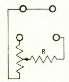
Potentiometer ratios can be related to angular rotation. Bridge reads  $R \times (1/ratio)$ .
