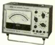
VOLTAGE RANGES 3 $\mu$ V, 10 $\mu$ V, 30 $\mu$ V, ... 1kV. Acc. = 1% = 1% f.s.d.  $\pm$  0·1 $\mu$ V, LZ & CZ scales. Noise < 0·5 $\mu$ V p - p on 3 $\mu$ V range. Drift < 0·7 $\mu$ V/°C & < 0·7 $\mu$ V/day. Input res. > 1M  $\Omega$ / $\mu$ V up to 10mV, >10kM $\Omega$  on 30mV to 1V, 100M  $\Omega$  above 1V.
