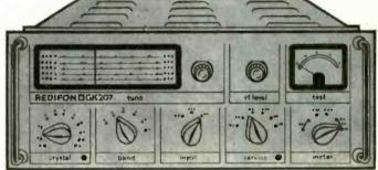
GK 207: 10 spot channels; manually tunable output circuits allow allocated channel frequencies to be changed rapidly by plugging in new crystals, without having to realign any pre-set circuits
