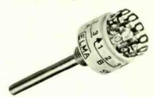
standard torque setting is 200 gm/cm; 400 and 600 gm/cm can be supplied to order. A ceramic wafer and gold-plated stud contacts are used. Contact resistance is better than 5mQ and wafer insulation better than  $10^{12}\Omega$ . Switching capacity is up to 1A. Radiation Components Ltd, 76 Crown Road, Twickenham, Middlesex. WW 309 for further details
