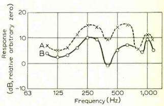
Fig. 5. Speaker moved to unsymmetrical position in room (warble tone).
