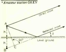
Fig. 1 When a horizontal aerial is erected at a height h over level ground, its image B is an antiphase. The direct and reflected waves are in phase at a distant point when  $BC = \lambda / 2$ , i.e. when  $2h \sin \theta$  $\theta = v/2$  where  $\theta$  is the angle of radiation.
