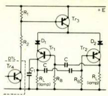
suitable are: diode IN4148 (G.E.); transistors (Ferranti plastic 'E' line) ZTX 500. B. L. HART,
