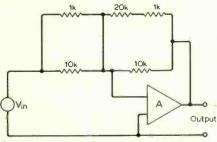
Fig. 3. Unity-gain version of Fig. 2 omitting  $R_1$ ,  $R_2$  and  $R_3$ .
