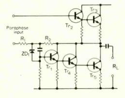
Fig. 1. Symmetrical output stage using only n-p-n transistors.
