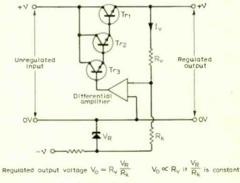
Fig. 1. A conventional stabilized power supply.
