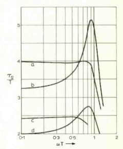
Fig. 18. Normalized group delay of Butterworth and approximately linear-phase filters.
