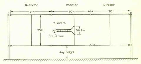
Fig. 7 Low-angle aerial for 7MHz. Height not critical. Reflector and director tunable, by adjusting length of verticals or of the lower horizontal wires. Dimensions approximate.
