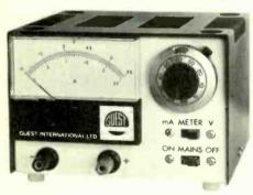
ability. A built-in meter enables the output voltage or current to be monitored. Ripple noise is less than 0.5mV pk-pk and overload protection limits the output current to 110% of maximum. Reset is automatic. The model 606 is available in current ranges from 0-500mA up to 0-2.5A. Dimensions are 156 × 152 × 102mm and prices from £34 15s to £42 15s. Guest International Ltd, Nicholas House, Brigstock Road, Thornton Heath, Surrey.
